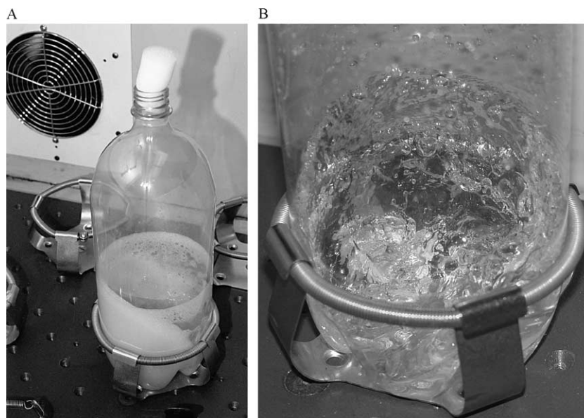
Fig. 1. Two-liter PET bottles as culture vessels. (A) A culture of E. coli expressing a heterologous protein in a 2-liter PET bottle. The medium, 250 ml TB, was not sterilized, but the presence of ampicillin and kanamycin prevented the growth of other microbes during the time required for expression of the target protein. The culture was agitated at 250 rpm. (B) Close-up view of a bottle containing 250 ml water, agitated at 250 rpm, to illustrate the effective aeration provided by the notches in the base of the bottle.
