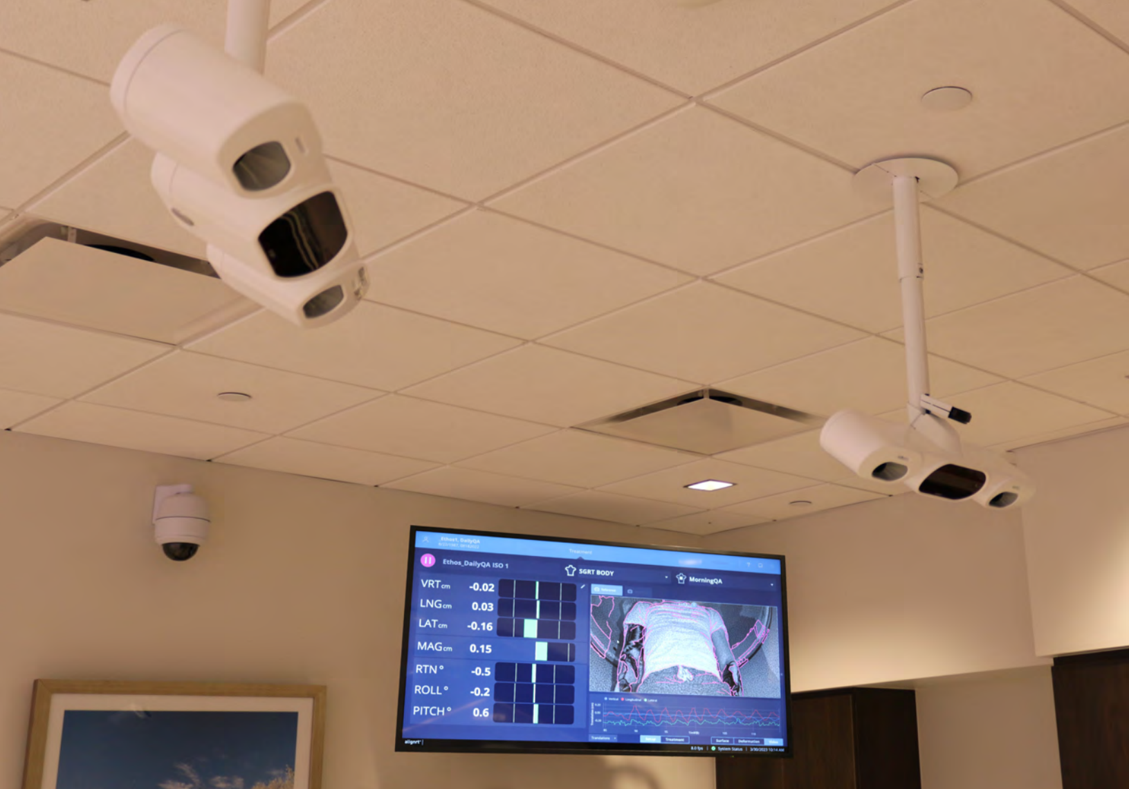
Surface-guided radiation therapy technology includes three ceiling-mounted cameras and a screen for motion management.
