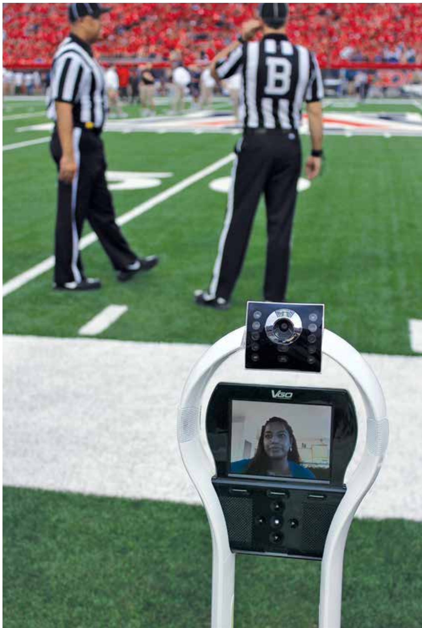
A "doctor" robot stands on the sidelines at a football game, with a remote health care specialist ready to evaluate injured players.
