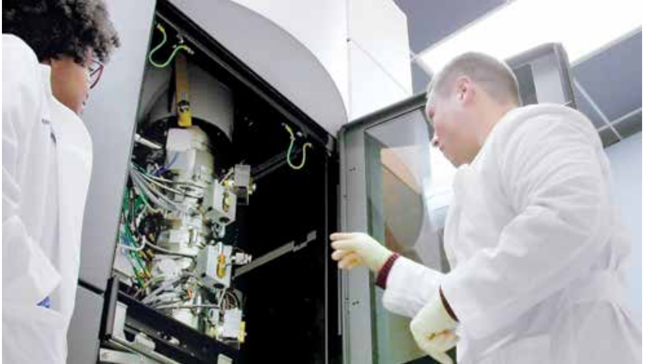
Daniel Stoddard, a Core Facilities Manager, shows the Titan Krios cryo-electron microscope to graduate student researcher DaNae Woodard.
